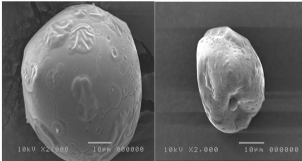
Figure 1. Scanning electron microscopy micrograph of encapsulated sesame oil powder at x2,000.
